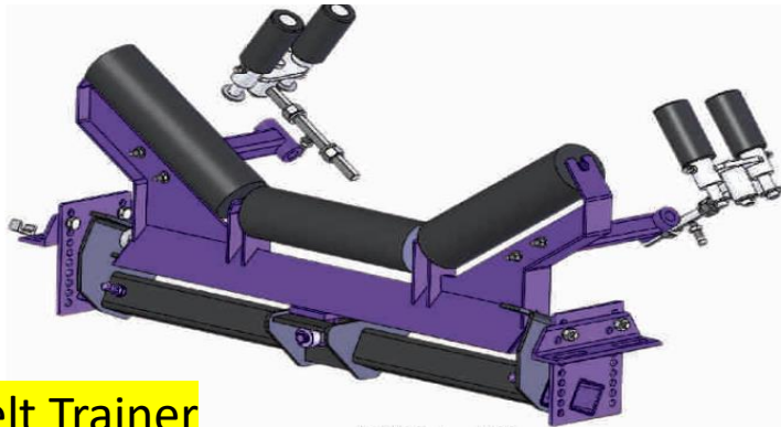
Belt running in center position without any drift or material spillage
